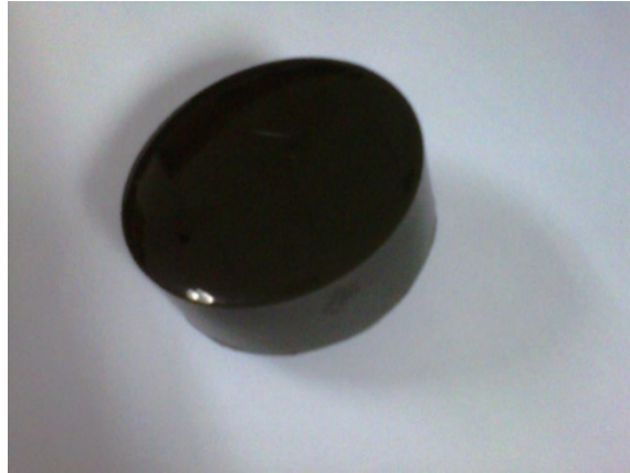
Figure 9 Polyurethane matrix composite with waste abrasive slurry reinforcing filler
